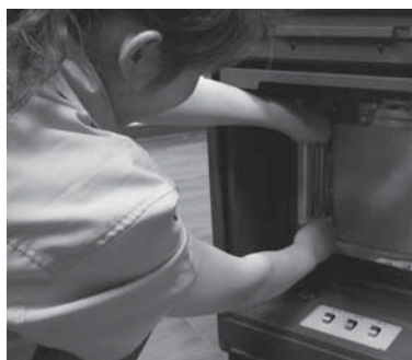
6-6 Replace the UV Lamps
