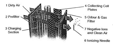
Dirty air is drawn in through the front grill and passes through a 4-Stage filtering system.
